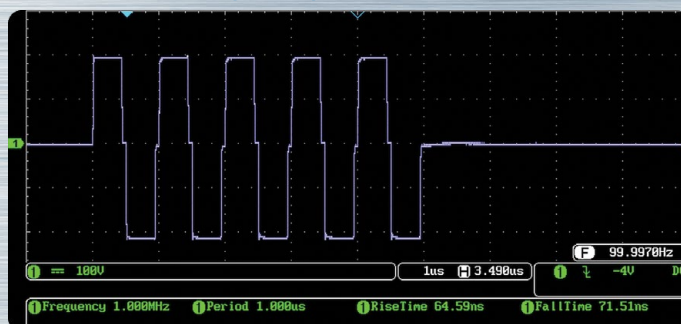
Scalable burst excitation pulse sequence ±200 V
